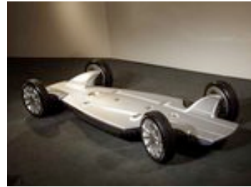
Figure 3 The GM AUTOnomy concept car consists of an undercarriage containing the hydrogen fuel cell. The basic shape and layout of today's car is heavily influenced by its source of power. Including the mode of propulsion in a minimal undercarriage provides new levels of freedom in design.
